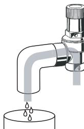
**i** If there is a risk that the discharge line becomes clogged or can freeze, interrupt the discharge line, e.g. by a funnel. The discharge line of the funnel must have twice the cross-section of the safety valve intake
