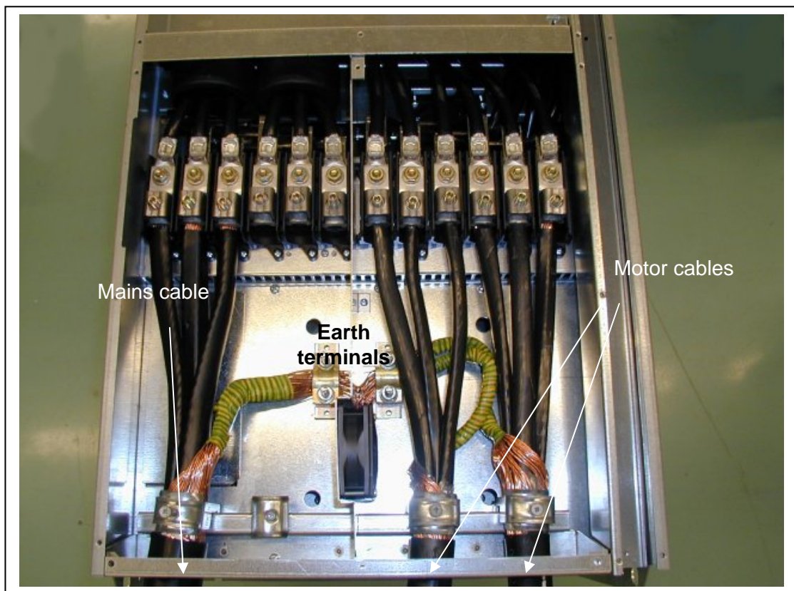
Figure 6-19. Cable installation in NX, FR9
